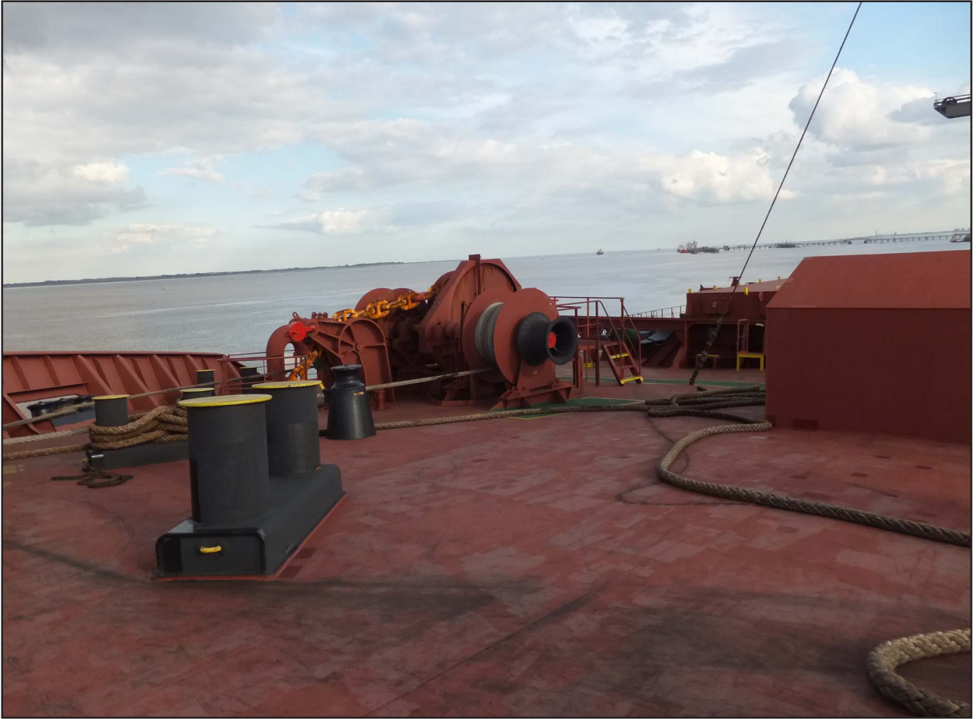
Figure 6: Forward mooring arrangement on Wah Shan
